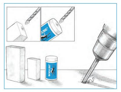
lubricant. Because minimal quantities are used and consumed for the most part in the machining process, BOELUBE Solids produce near dry workpieces and chips with little or no clean-up or related costs and no disposal costs.
