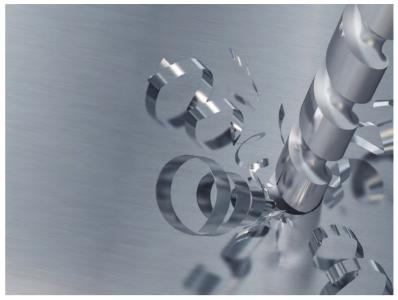
MQL lubricants can also be formulated into paste form - BOELUBE Pastes. In MQL machining the goal is high efficiency, which is achieved as a result of using a minimal quantity of lubricant. Because minimal quantities are used and consumed for the most part in the machining process, BOELUBE Pastes produce near dry workpieces and chips with little or no clean-up or related costs and no disposal costs.
