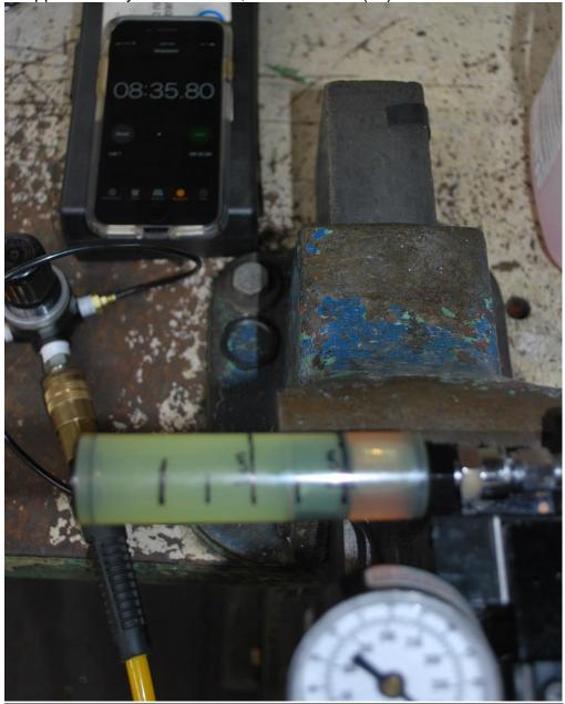
The usage of a Zephyr ZT4000 positive feed drill at 2200 rpm, 0.006 feed rate, drilling 1" thickness of aluminum with  $\frac{1}{2}$ " drill bit diameter results in average drill time of 8-10 sec per hole. Thus, a full cartridge of 15 cc (ml), should drill between 77-97 holes at approx.1.17 ml/min.
