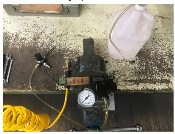
To simulate the positive feed drill working scenario the air pressure was regulated to 55-60 PSI and adjusted the amount of lubricant with Unist Piggyback portable cutter lubricant system.
