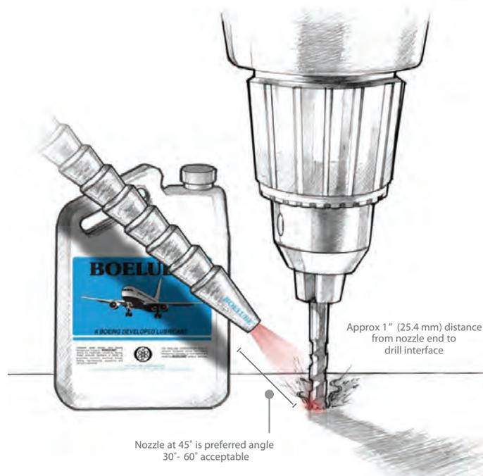
Using a coaxial supply of compressed air and lubricant to the nozzle, the nozzle directs BOELUBE® lubricant droplets in the compressed air directly to the cutting edge. The compressed air will help move chips from the tool cutting edge as the fine lubricant droplets form a thin film at the point of contact to reduce friction.
